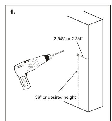
Choose desired height (ususally 36") on door for the knob. At this height mark the door 2 3/8" or 2 3/4" from door edge.
