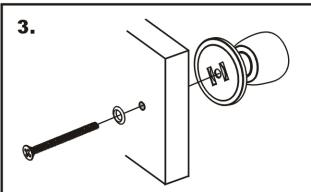
With bolt head and washer on inside of door, attach knob on outside.
