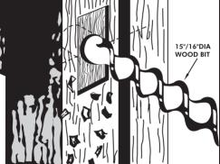
Drill 15/16" diameter hole 1/2" deep in center of mortise.
