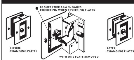
When it is desirable to reverse outside plates on lock assembly, firstremove machine screw on each side-change plates from side to side ( making sure that fork arm engages rocker pin ) and re-assemble.
