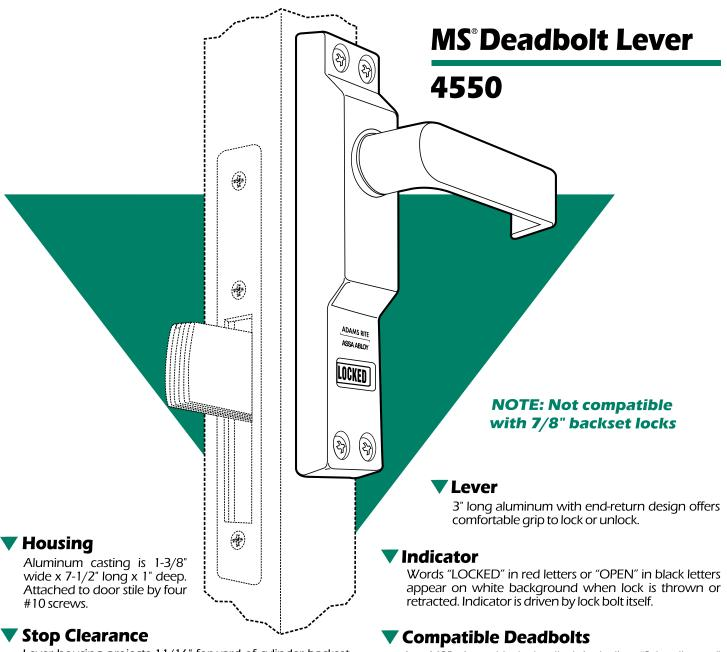
Lever housing projects 11/16" forward of cylinder backset centerline. Depending on height of door stop and width of door/jamb gap, it may be necessary to modify the stop to clear the housing. (For fin type stops, this is easily accomplished.) Hollow stops may preclude use of lever.
