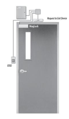
**Note:** Securitron's UL294 certification indicates that when the EEB is used with the XMS Motion Sensor, it meets the NFPA Life Safety Code 101 requirements for exit of access-controlled egress doors.
