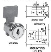
**APPLICATION** – C8701: for center drawers of metal desks. Fits special piercing of drawer front and selvedge (see drawing). C8896 is a specific replacement lock.
