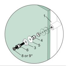
Install the interior handle onto the collars.
