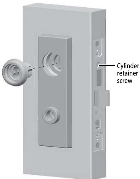
Figure 18b Installing the high-security cylinder
