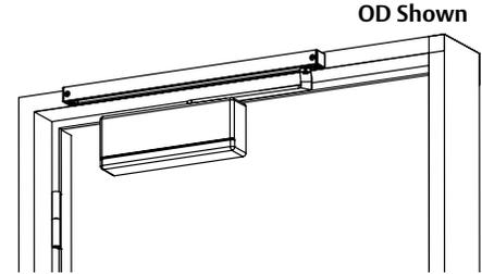
281 Track Type Application offers a number of options such as built in bumpers and holders. Along with its clean appearance, it is a favorite for many interior designers. It has the versatility of being mounted on either side of a door for the clean unobstructed appearance without the cost of concealed closers and tracks.
