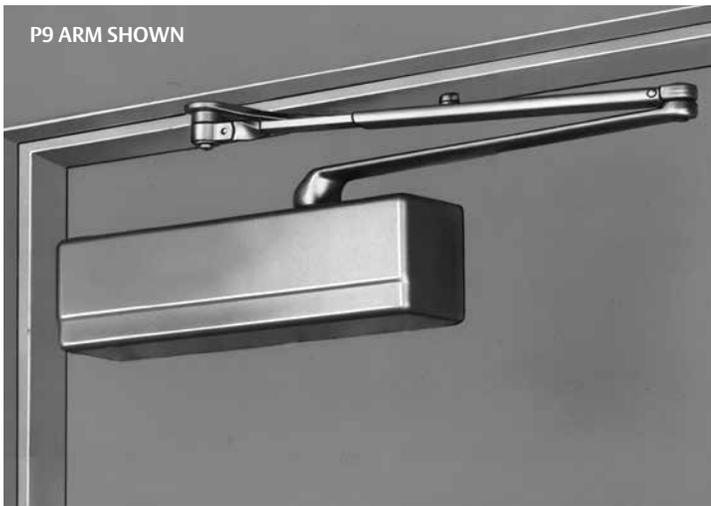
Parallel Arm Application – The 281 closer is mounted on the push side of the door. As the door opens, the closer swings with the door and gives full headroom in the door opening. Other advantages are that the closer arm does not project into the room, the frame can be quite narrow and the door can be swung open much further than in Top Jamb Applications. However, the closing force is not as great.
