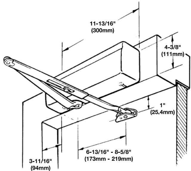
Top Jamb Application – The 281 closer is mounted on the frame face above the door. The foot is mounted on the push side of door. This application is for use on exterior doors opening out to protect the closer from the weather. The Frame Face must be at least 4-3/8". With the 281-B mounting plate, the rail must be at least 1-7/16" min.
