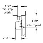
The push side application of the 421 cam closer provides the most aesthetically pleasing appearance of any surface mounted closer. With both the closer and compact track tucked under the door frame, the 421 closer in the push application almost disappears into the opening. In this application, the closer body mounts to the face of the door and the track mounts to the soffit under the frame. All cam action closers are equipped with a short track further minimizing the appearance of the closer.
