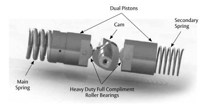
The SARGENT 421 is a revolutionary door closer that provides unheard of performance in track arm applications. The dual piston cam design provides high efficiency and smooth operation with the clean appearance of a track arm.
