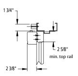
The pull side application of the 421 cam closer provides an aesthetically pleasing appearance with the functionality of pull side mounting. In the pull side application, the closer body mounts to the face of the door and the track mounts to the face of the frame. All cam action closers are equipped with a short track which provides superior door control with a clean appearance.
