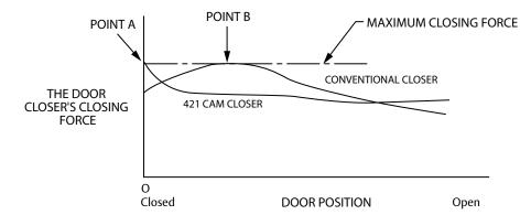
Point A - The Cam Closer has the maximum closing force at the point the door is closing.
