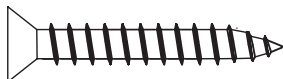
#12 x 1 1/2" Phillips Flat Head Sheet Metal Screw Use 9/64" Drill bit Also: #12 x 1"
