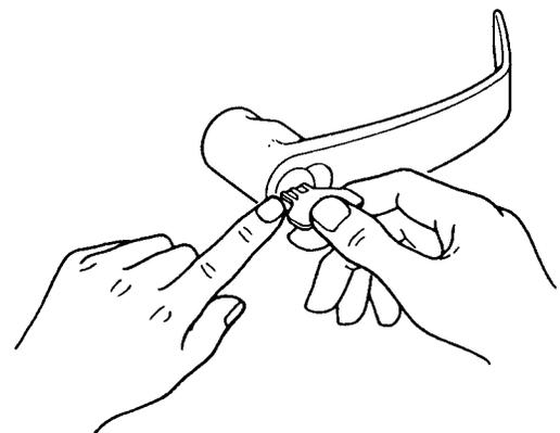
**NOTE:** FOR EASIER REMOVAL, HOLD CORE IN PLACE WHILE STARTING TO WITHDRAW KEY.
