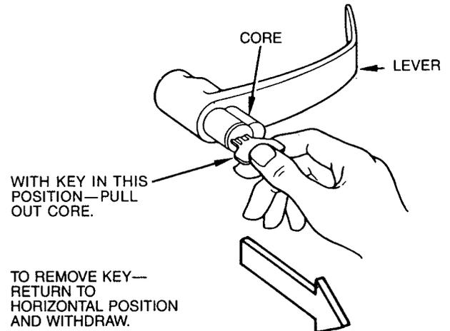
WITH KEY IN THIS POSITION—PULL OUT CORE.
