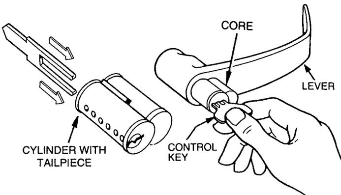
TO REMOVE KEY, RETURN TO HORIZONTAL POSITION AND WITHDRAW.
