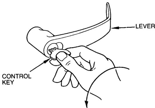
THEN INSERT CONTROL KEY AND TURN COUNTER-CLOCKWISE UNTIL STOP IS REACHED. (CLOCKWISE FOR BEST, ARROW, AND FALCON).
