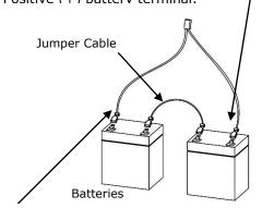
Connect black battery lead to the unused Negative (-) battery terminal.
