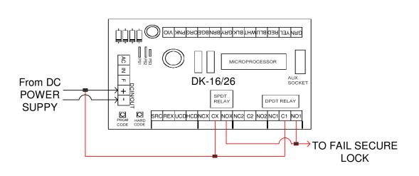
Wiring a DK-16 or DK-26 for HARD CODE Openings & Closings (with a Fail Secure Lock)
