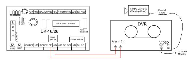
Wiring a DK-16 or DK-26 to Activate the Alarm input of Time Lapse Video Recorder or Digital Video Recorder (DVR) for a <u>Visual Audit</u> of Entries at the Keypad.
