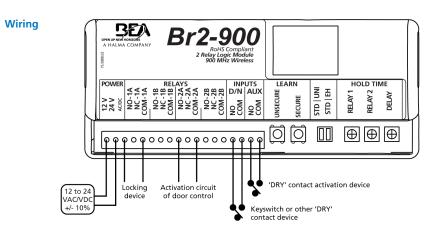
Relays 1 and 2 are DPDT: relays 1A and 1B fire simultaneously and relays 2A and 2B fire simultaneously.
