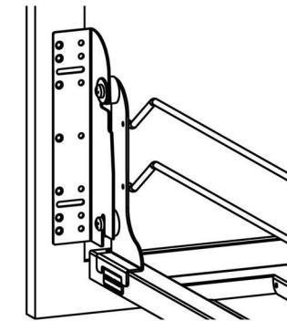
**5) Apply double stick tape to the door brackets. Attach cabinet door to the brackets while trying to keep door level. Don't worry if it is off a little, this can all be adjusted. Double stick tape will hold the door in place while you crew the brackets to cabinet door.**
