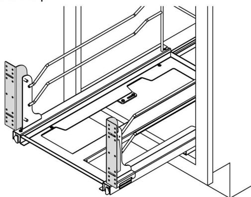
**4b) Each cabinet door is different, make sure the door bracket lines up with the thick portion of the cabinet door.**
