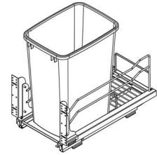
1) Install the side skirts to the slides as shown. Be sure to securely engage the rear of the slide under the metal tab before installing the phillips head screw at the front of the slide. Be sure the slide feet are pointed inward as shown.
