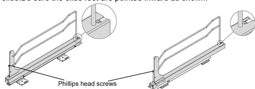
2) Install the main chassis to the slides as shown using the 4 machine screws provided and install the crossbar.
