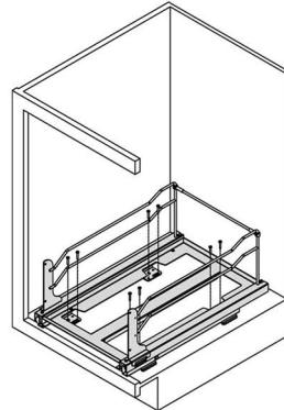
**4a) Attach the door brackets to the outside of the L-brackets using the (4) provided screws. The screw with the washer goes at the top.**
