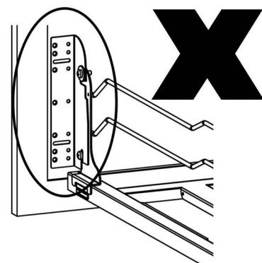
**4c) Plastic spacers are provided if the door brackets need to be extended further to reach the thick portion of the door.**
