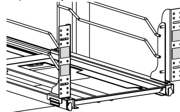
**6) Using provided wood screws, secure brackets to cabinet door.**
